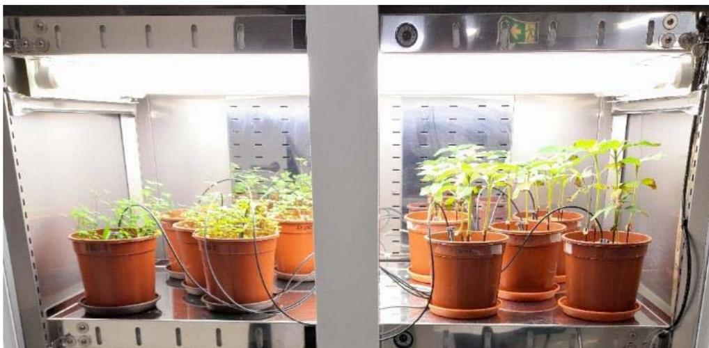
**Figure 1:** The setup for the plant cultivation inside the climate chamber. The lucerne is on the left and the sunflower on the right. A hose connects each pot to the Hoagland solution supply in the center.
